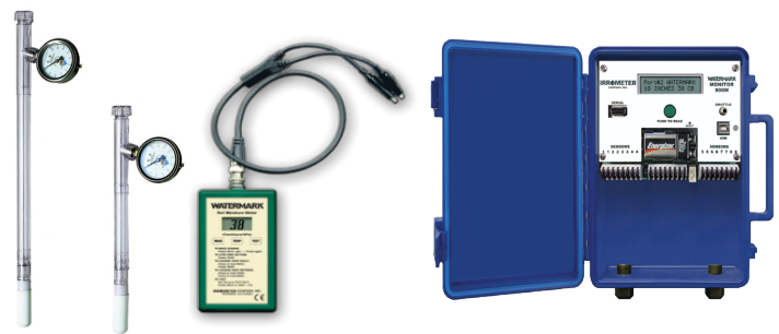
Figure 1: Tensiometers with gauges, a handheld meter, and a datalogger (image credits: Ele International and Irrrometer)
