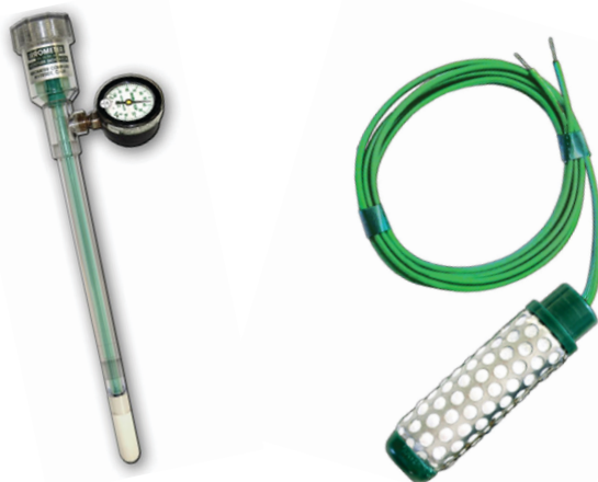
Figure 1: Ceramic-tipped tensiometer (left) and granular matrix sensor (right). Image credit: Irrrometer
